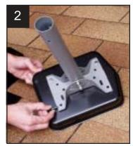
2) Bolt Deck Adapter to either Commdeck or Retrodeck using (4) Cap Bolts provided with Commdeck and Retrodeck hardware package.
