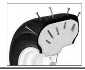
Cross section of filled NFL (Non Flat Lite) Tire with nails
