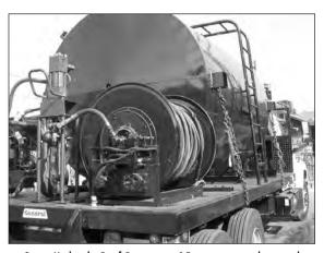
Graco Hydraulic Roof Rig powers 15 gpm pump & hose reel
