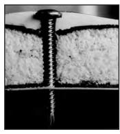
CROSS SECTION of insulation with plastic Stress Plate 750605
