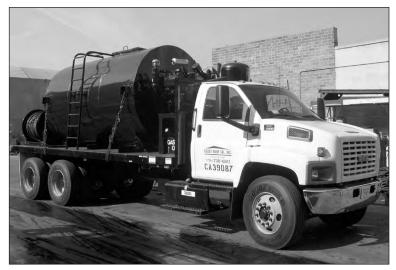
Emulsion tanker, set-up for spraying monoform systems
