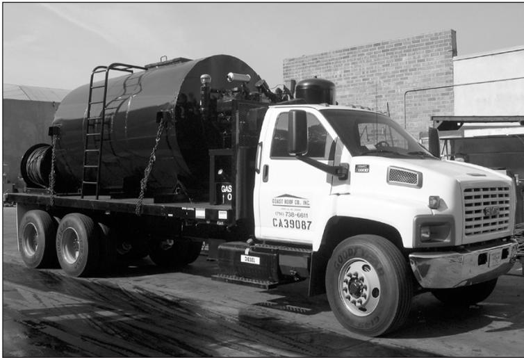
Emulsion tanker, set-up for spraying monoform systems
