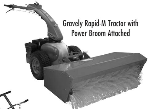
Gravelly Rapid-M Tractor with Power Broom Attached
