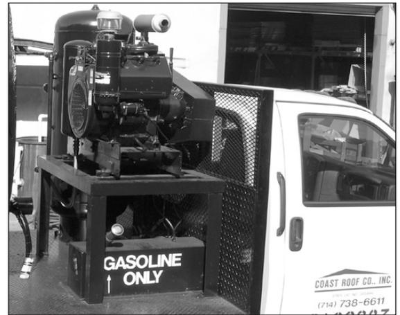
30 hp air compressor with 120 gallon vertical reservoir
