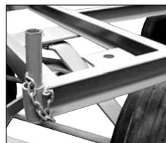
4 corner pin pockets accept pins to hold roll goods & prevent rolling off trailer.
