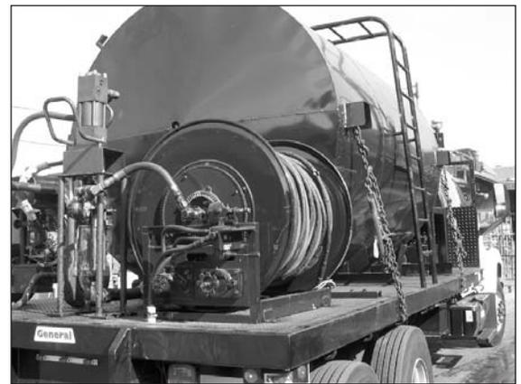
Graco Hydraulic Roof Rig powers 15 gpm pump & hose reel
